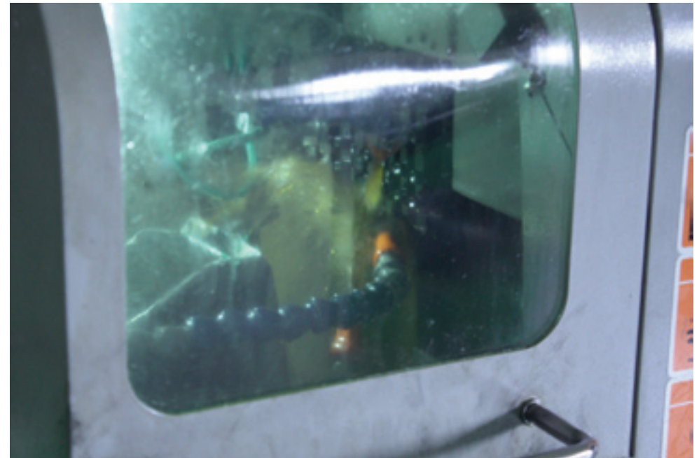
Fig. 12 Machining Cutting Lube's dispensing Form
