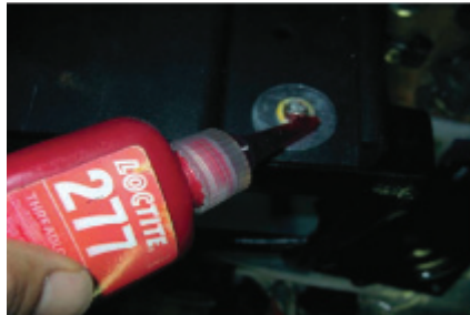
Fig. 79 Sealant adhesive to fill the Bolt and Nut top region
