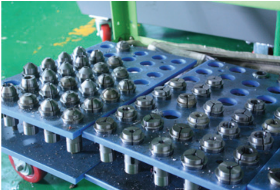
Fig. 5 Guide Bush and Chuck Slot for Gap Adjustment according to Diameter of the materials
