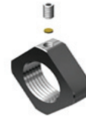
Fig. 80 Set Screw is fastened to prevent Nut reversion
