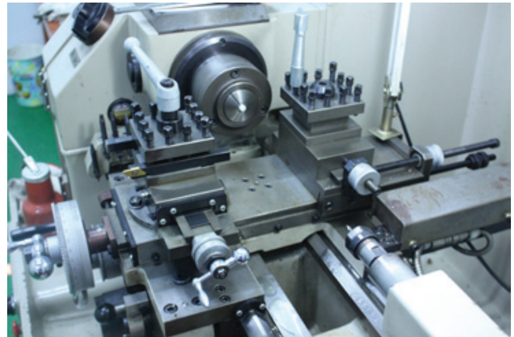
Fig. 15 In manufacturing the Taper the angle of the Tool Rest Head in Manual Lathe is adjusted and more precise (than NC) manufacturing can be done.
